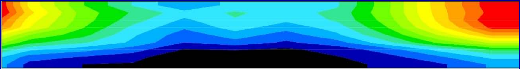
Measured temperatures, horizontal duct at reactor inlet
